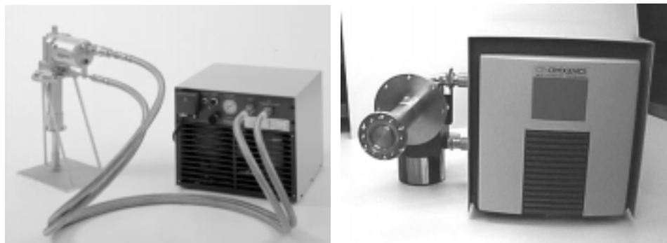
Fig. 45 (left) A 19 in. rack-mountable Leybold “4.2LAB” 2-stage Gifford-McMahon cryocooler delivering ¼ W of lift at 4 K for 2 kW input power. (right) A CTI single stage Gifford-McMahon cryocooler delivering 60 W lift at 60 K with a no-load temperature of 45 K.
